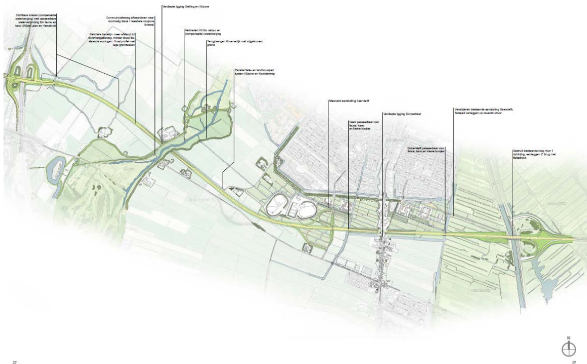
Image 6: Hemskeerk alternative, showing the layout of the proposed alternative with the three nodes of intersections, as well as the mitigation measures.
